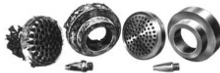
Extruder parts before and after being cleaned in a Techne Industrial Fluidized bath
