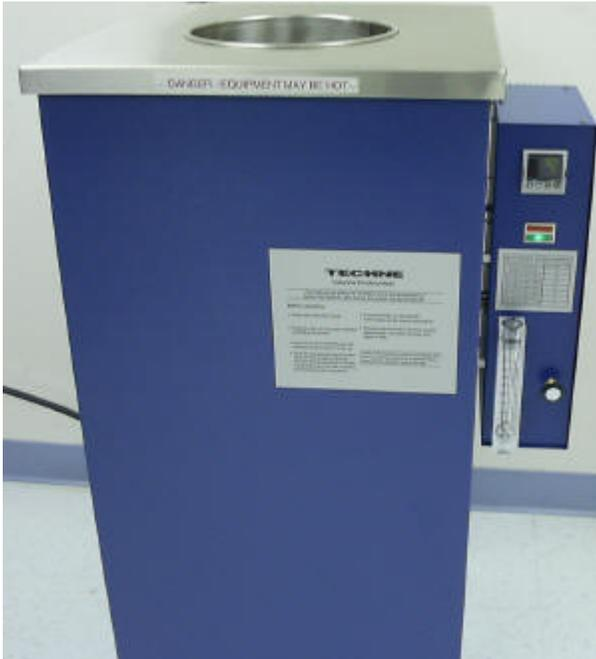
**NEW FEATURE >>** The IFB-51 and IFB-52 baths now incorporate an acrylic flow meter and fine adjustment valve for precisely setting, measuring and controlling the Fluidization air. This new feature greatly improves the stability to  $\pm 1.0^{\circ}\text{C}$  and accuracy to  $\pm 10.0$  throughout the operating range. A label above the flow meter shows the factory suggested settings to use. See a close up image of the [new Flow meter](#).
